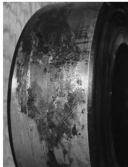
Fretting on the outer ring due to out-of-round housing bore.
