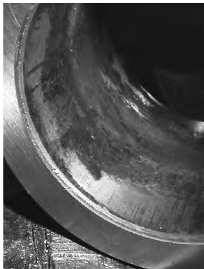
Fretting on inner ring due to out-of-round shaft.
