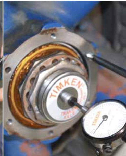
Proper bearing adjustment plays a major role in maximizing bearing service life. If bearings are adjusted with too much internal axial clearance (end play) or too much internal load (preload), the life of the bearing and other wheel-end components may be shortened.
