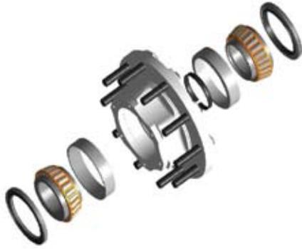
the nut acts to retain it on the spindle. This type of wheel-end system cannot be serviced in the field. The entire system will need to be replaced. You cannot replace separate components.
