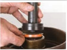
The grease seal must be replaced when it leaks or when bearings are being repacked or replaced. Install the inner bearing cone assembly in the hub, then the new seal. Make sure the seal lips are pointed in the right direction following the vehicle
