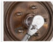
Use a torque wrench to tighten the adjusting nut to 50 ft. lbs. while turning the rotor. Back off the adjusting nut 1 full turn. Then retorque the nut to 10 ft. lbs. while turning the rotor. Next, back off the adjusting nut ¼ turn. Lock the nut with a new cotter pin.
