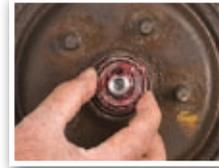
Slide the rotor/hub assembly back over the spindle, being careful not to damage the seal against the spindle. Pack the outer bearing cone assembly with grease following the procedure outlined in the first paragraph of Step 4. Install the outer bearing cone assembly, washer and adjusting nut on the spindle.
