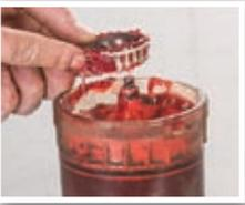
Pack the inner bearing cone assembly with grease. A mechanical grease packer is recommended.
