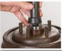
Use a cup driver or mild steel bar to press or drive the new inner cup and outer cup into the hub/rotor assembly until they are solidly seated against the hub shoulders. Be careful not to damage the cup surfaces. Never use a bearing cone assembly to drive a cup.
