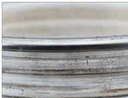
Cup spinning - Loose cup fit in a rotating wheel hub.
