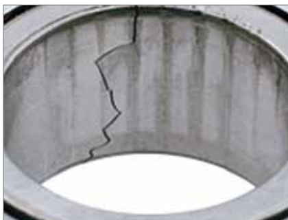
Cone bore damage - Fractured cone due to out-of-round or oversized shaft.
