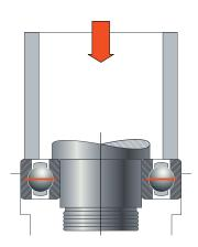
bore. Note that in this scenario the shaft does not rotate and is loose fit in the inner ring, while the outer ring is tight because it rotates in this application.
