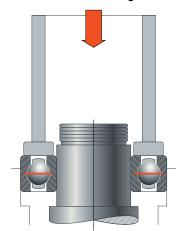
and/or housing. Note that in this scenario, the shaft is already in place. Attention must be given to any bearing on the other end of the shaft to ensure it is properly supported and not damaged. Make sure there is no contact (or any damage) with the bearing cage. Any indication of a bent bearing cage renders the bearing unusable.
