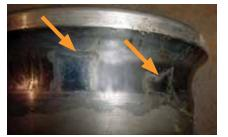
Chemical reaction of grease and moisture in a prolonged static condition resulting in pitting and corrosion. A 'witness mark' is generated at each ball location on the inner race.
