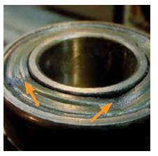
Seal damage due to improper installation procedure and/or tools.
