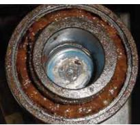
Lubrication characteristics of the grease are compromised by water ingress.
