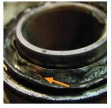
Distorted seal due to interference with adjacent mating parts.
