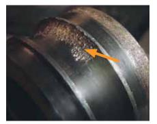
Geometric stress concentration (GSC): spalling from misalignment, system deflections or heavy loading.
