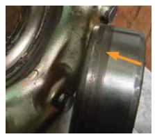
Bearing supported by only one-third of its outer ring width within housing.
