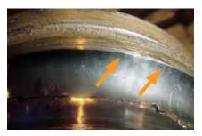
Damage from shock or excessive loads.
