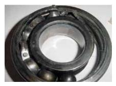
Metal cage damage due to misalignment or excessive speed.
