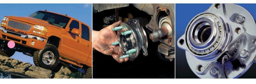
Timken continues to lead the hub evolution by manufacturing assemblies that are uncompromised in quality, reliability and consistency. Proper hub removal and installation procedures can enhance the performance and life of hubs, axles, wheels, brakes and other components. Following are general recommendations for removing and installing hub assemblies.
