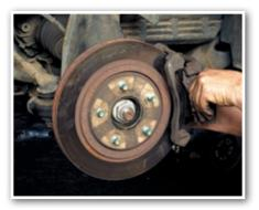
3 Remove the axle nut using an axle nut socket. Use the vehicle manufacturer's instructions regarding nut replacement.
