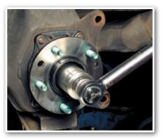
5 Replace the brake rotor and brake caliper. All components should be clean from debris and burrs.
