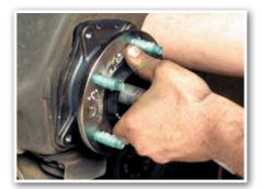
2 Torque the knuckle-bearing mounting bolts to the vehicle manufacturer's specification using a torque wrench. An impact wrench is not recommended because it does not reliably impart the proper torque.
