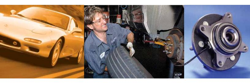
Signs of a worn wheel hub bearing vary in severity. Some may be difficult to detect, leading to damage before corrective action can be taken. The time frame in which damage occurs is linked to driving conditions and/or the mechanical practices that were followed at installation. Noise is a classic sign of a bad wheel bearing or wheel hub bearing. Here are some indicators of a worn wheel hub bearing or other wheel-end damage:
