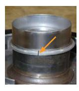
5) Fill deeply scored grooves with a thread repair compound. Place the sleeve onto the shaft before the compound hardens. The
